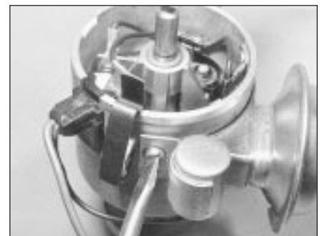
2.21 Extracting vacuum diaphragm unit screw
