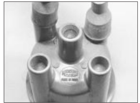
11.7 Distributor cap HT lead markings
