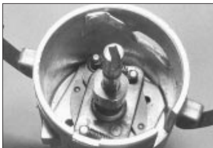
7.13 Marelli distributor centrifugal weights and springs
