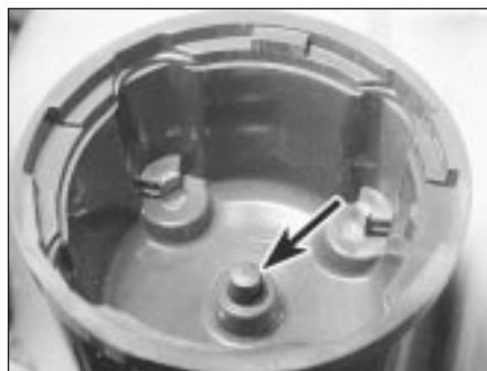
2.16 Interior of distributor cap showing carbon brush
